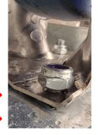
If the locknuts are not installed correctly, clearly mark and isolate the trolley base to ensure that it cannot be used.
